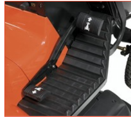
Hydrostatic gear box - no gear changing
