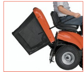
Easy grass box emptying by telescopic lever
