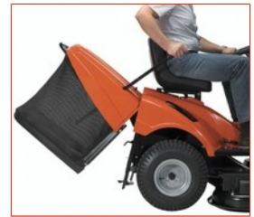
Easy grass box emptying by telescopic lever
