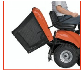
Easy grass box emptying by telescopic lever
