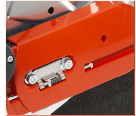
Easy belt tensioning with screw driver
